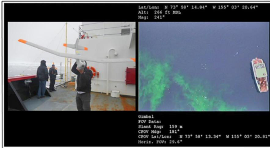
Shield crew dispersing the dye. The left side of Figure 2 shows an image of the Puma just prior to one of its flights during Arctic Shield. The right side of Figure 2 shows Puma visible imagery of the dispersed dye along with aircraft position and attitude information.
