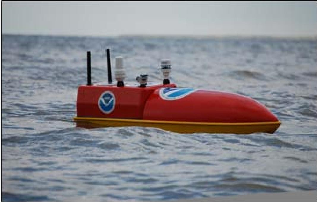
EMILY, a 65-inch watertight craft, is one of the newest of NOAA's hurricane research platforms. Outfitted with a satellite link, camera, battery and gasoline motor, and a variety of sensors, EMILY will collect sea-level data from within a hurricane beginning with the 2012 hurricane season. Credit: Hydronalix Inc.
